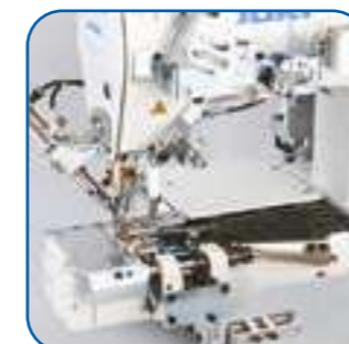
Pneumatic type needle thread / looper thread trimming device.
