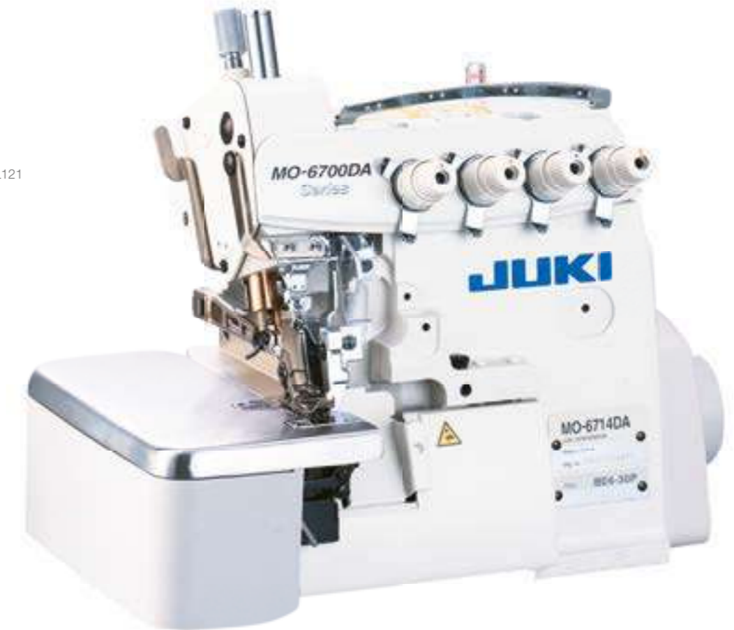
Gathering - MO-6714DA-BE6-327/S162 (S162: Swing-type gathering device, manual-lever operated)
