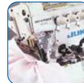
Gathering - MO-6714DA-BE6-327/S162 (S162: Swing-type gathering device, manual-lever operated)
